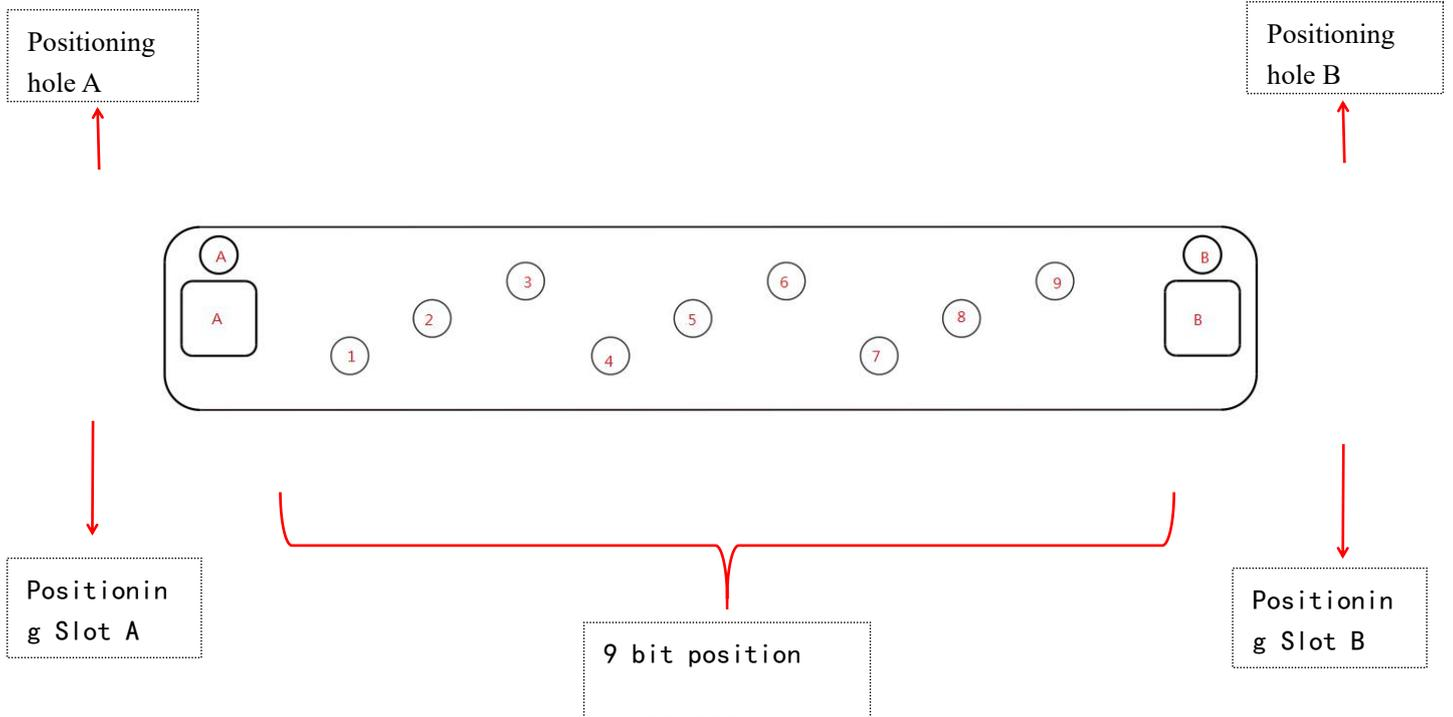
CutterServer Auto changer bit page, select shifting correction(router bit library will open automatically).
