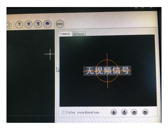
Check the CCD cable connection from CCD to PC.
