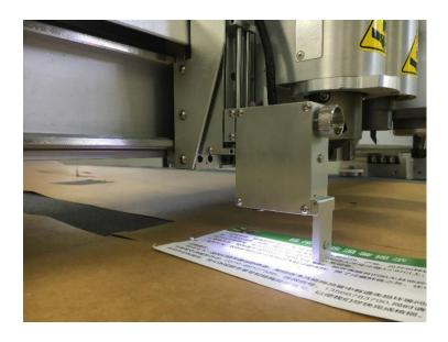
If the image is still not clear, adjust the CCD focal spot(focus) shown in the below picture.
