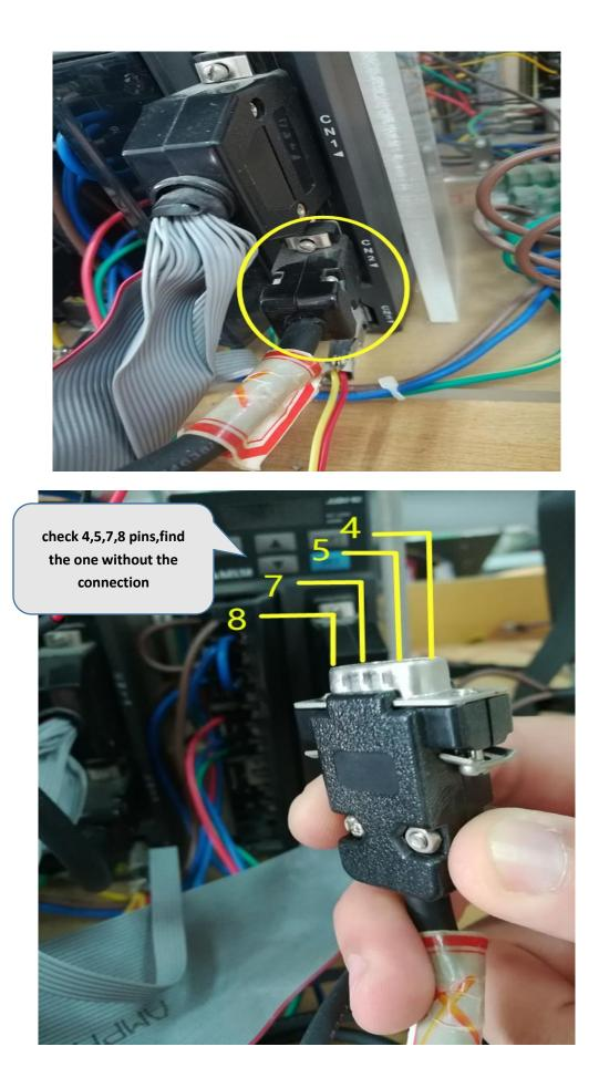
(3) If no driver with error AL-011, check the B board. For BK model, please check D1 D2 LED. For BK3 model, please check ZH\_A ZH\_B. If the LED dose not flash when you rotate the head, it means the B board is broken.
