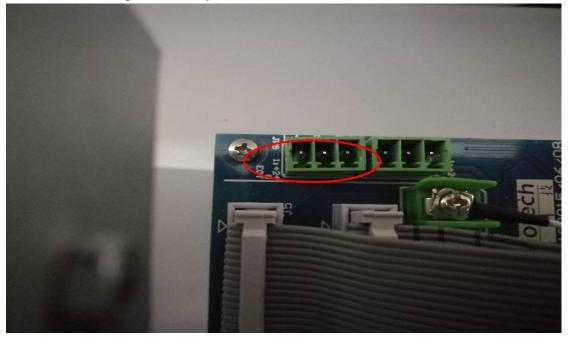
**3.** If the EOT always oscillating, check the B board EOT plug between blue and black, when you didn't select EOT, the voltage should be zero. If not mean your B board is broken.
