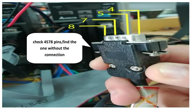
(3) If no drive error is reported, check the B board. BK3 check ZH\_A ZH\_B, if the LED does not go out when you rotate the head, means the B board is broke.
