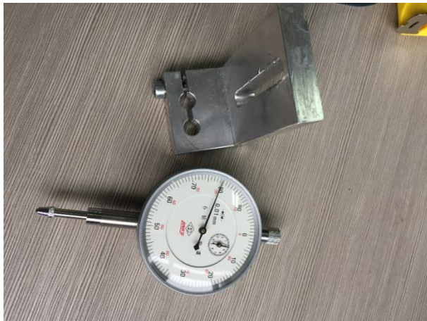
Dial Gage (used for adjusting the machine table level)
