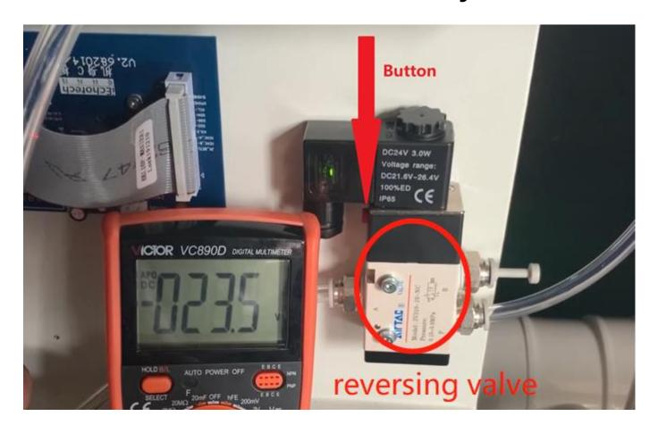
If it can not work manually, check the air input. If the air input is good, then the reversing valve part is broken.
