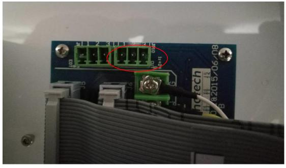
**3.** If the DRT/PRT always rotates, check the B board DRT/PRT plug between blue and black, when you didn't select DRT/PRT the voltage should be zero. If it not means your B board is broken.
