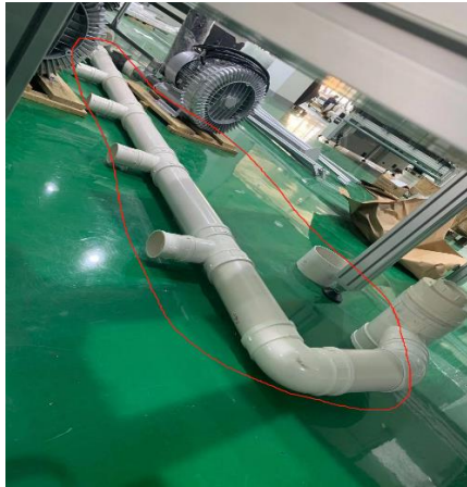
Combine the PVC tube outside the machine, totally 4 unit.
