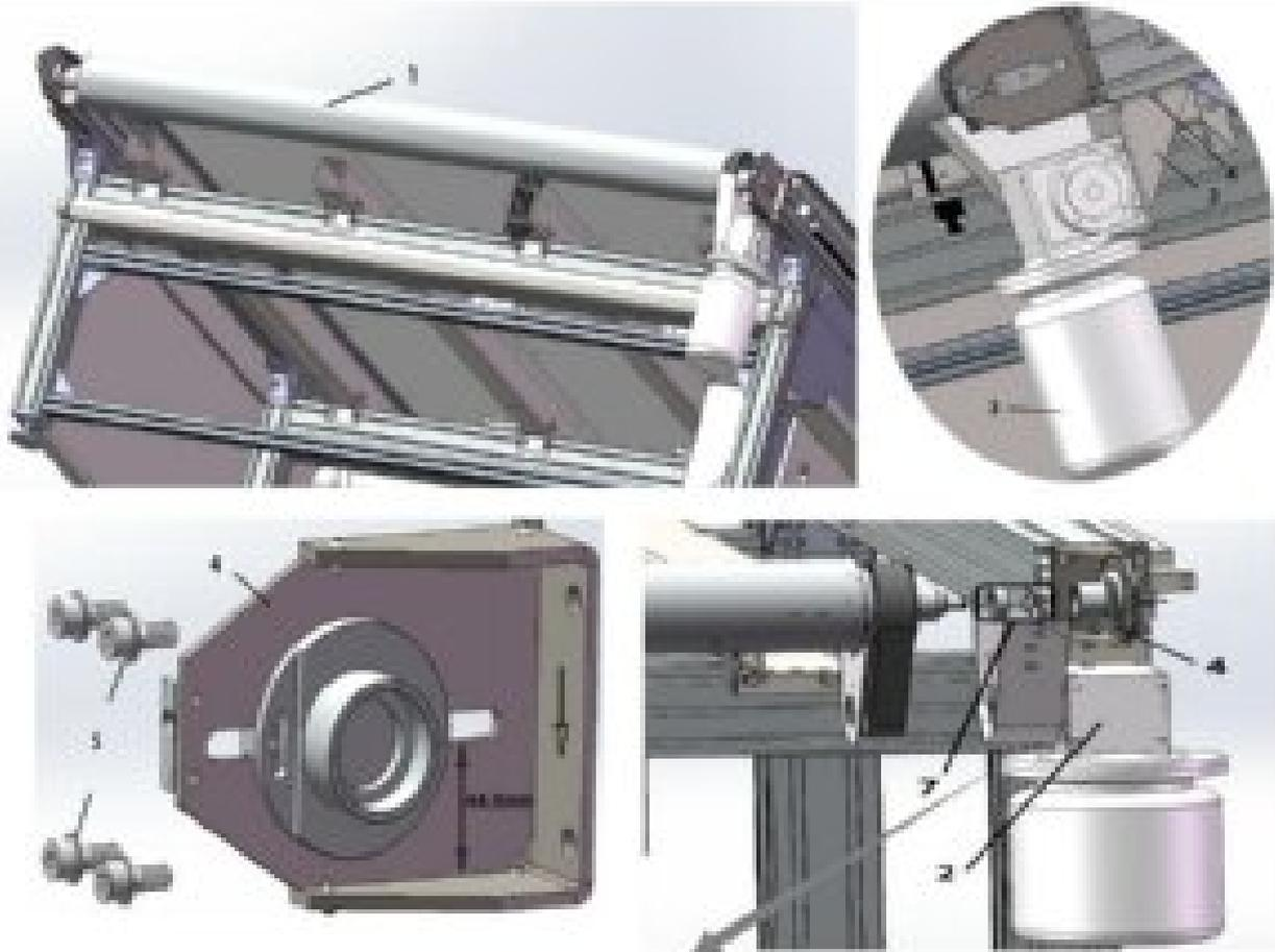
installing steps of this parts : 1. motor bracket support(2) 2. mounting plate(4)
