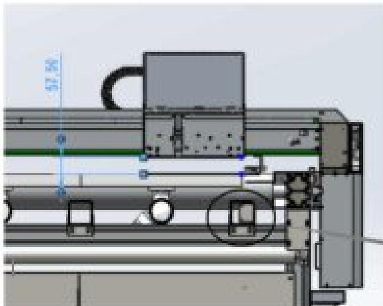
Measure the distance from the bottom of the module carriage to the surface of the aluminum platform with a steel ruler is  $57.5\text{mm} \pm 0.5\text{mm}$ .
