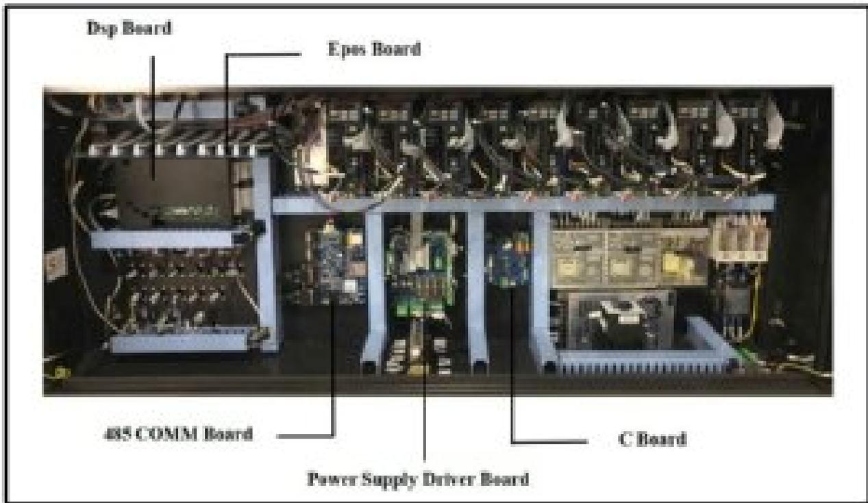
■ Boards positions on machine (behind the cutting head device)
