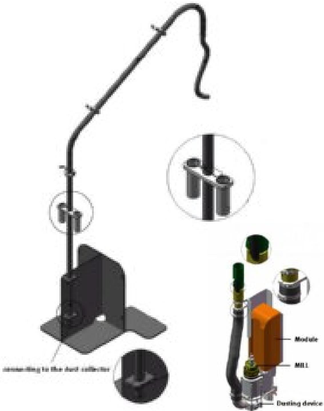
**Connect cables in the milling device support**
